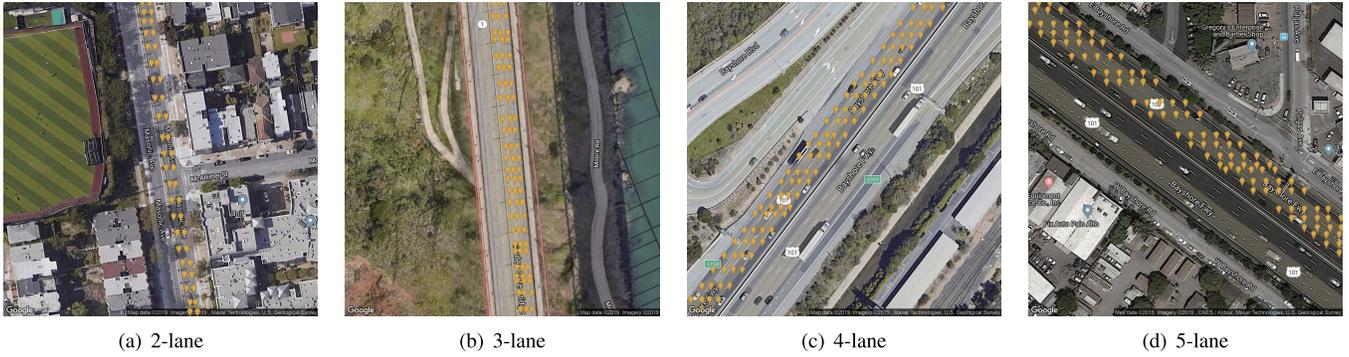
Fig. 14. Marking of lane centerline on Google map when the confidence coefficient of road boundaries is set as 95%.
